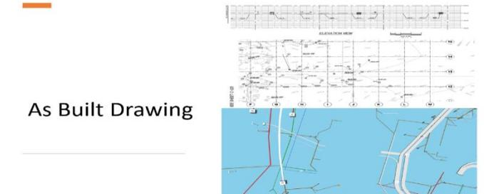
After Installation of Utility networks based on BIM drawings, Site team use to mark-ups the updates and changes in the plans based on the actual installation in site. Based on the site mark-ups, we create as built 3D model & Drawing and prepare the as built set for project hand over and record.
