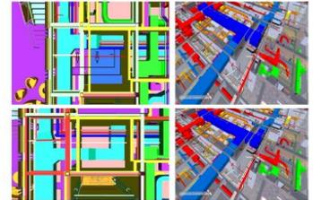
We generate a coordinated BIM model after resolving the clashes among all disciplines – Architectural, Structural, Concrete & Mechanical.
