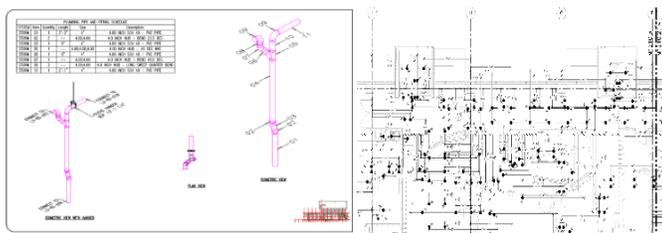
**Shop Drawing:-** Our cad team produce the shop drawing from CAD design drawing to incorporate the details of all fitting, accessories, details including as follows. Drawings shall be indicative of actual equipment purchased and shall show all offsets, transitions, fittings, dampers, valves, hanger locations.
