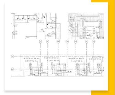
Penetration, Sleeve Drawings are required before a contractor can start pouring concrete on the site. Penetration Drawings are created from the coordinated BIM model after alignment with the architectural grids. Our experienced team keeps the necessary clearances for the penetration as per the contract documents and Specification.
