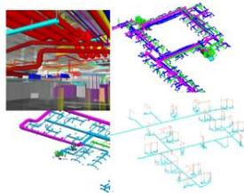
We are specialize in the virtual construction of 3D models @ LOD 400 of Mechanical systems i.e. ducting, piping with fitting including all valves & accessories with all associated equipment's and fixtures. We produce 3D Models based on contract drawings, technical specifications, and manufacturer details to client standards.
