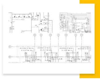
Penetration, Sleeve Drawings are required before a contractor can start pouring concrete on the site. Penetration Drawings are created from the coordinated BIM model after alignment with the architectural grids. Our experienced team keeps the necessary clearances for the penetration as per the contract documents and Specification.
