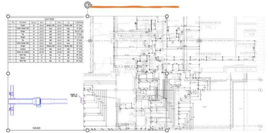
D & D produce the Spool drawings, Hanger & insert drawing with proper co-ordination of model and placing the hangers in line with specification. Hanger drawings shows the actual location of hangers with proper dimension from wall or grid. Insert are position of hangers insert points and D & D produce the proper insert drawing coordinating with actual hanger location in the model.
