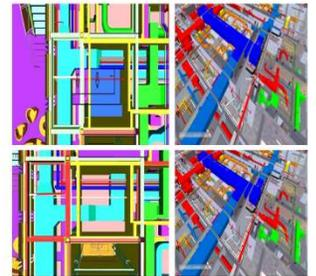
We generate a coordinated BIM model after resolving the clashes among all disciplines – Architectural, Structural, Concrete, Mechanical, Electrical, Hydraulic, Fire Protection, etc.
